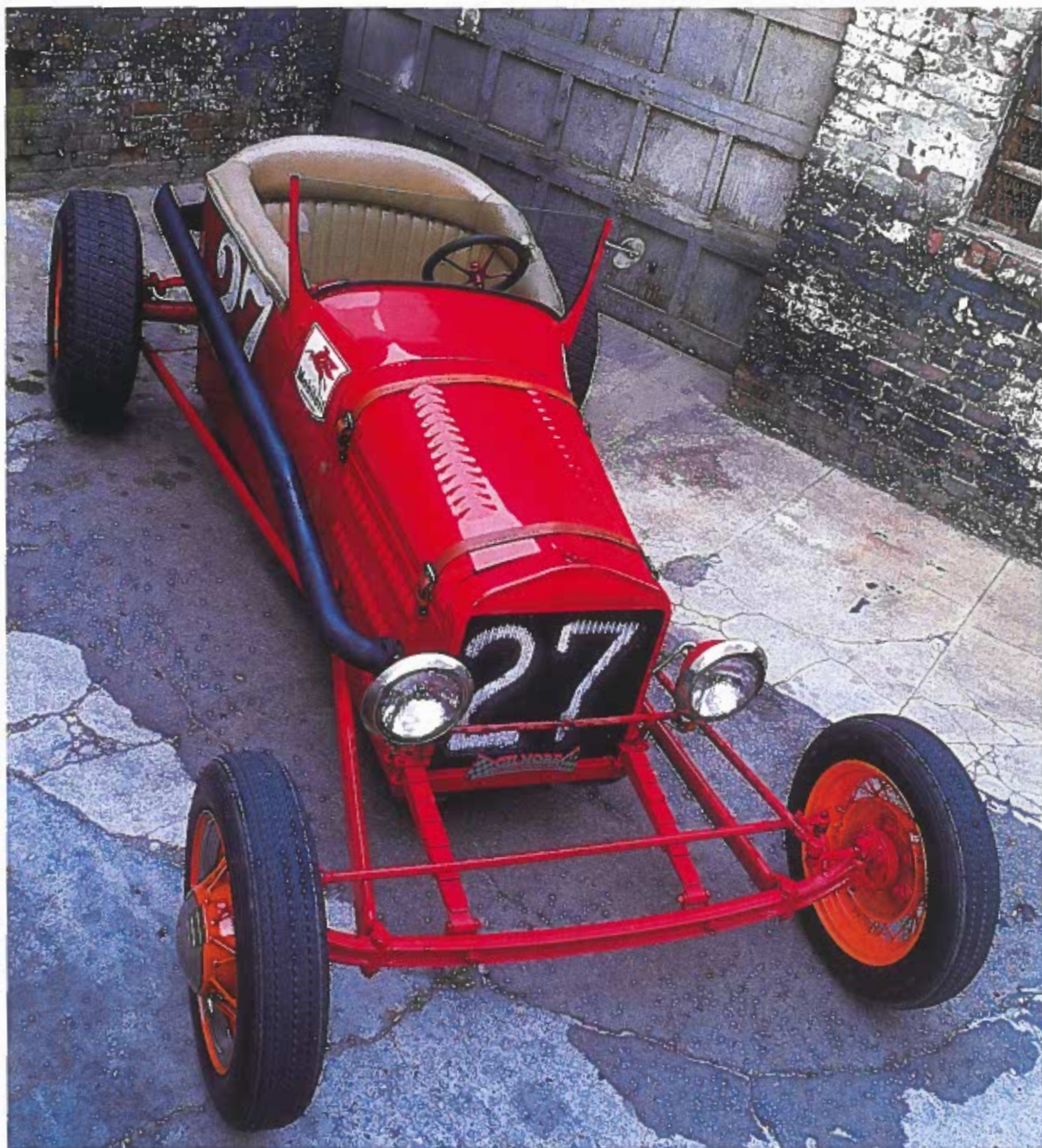
Howard Holman bought this modified-T roadster for several thousand dollars in 1990, then he spent several months and a few more bucks restoring it. The suicide front end was common on modified roadsters. Unlike early modified roadsters that usually were powered by Ford fours, Howard's bobtail T has a late model Pontiac four-banger engine.
